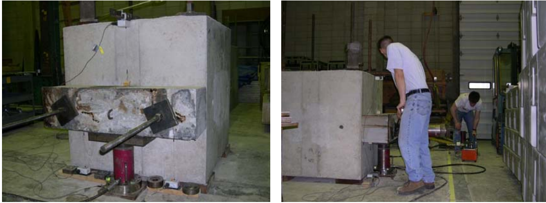
(a) Assembled precast paving notch system (b) Application of PT force Figure 2. Photographs of the assembled precast paving notch system and the application of PT force.
