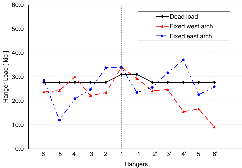
FIGURE 6 Hanger forces for both arches of the 44th Street Bridge after adjustment.
