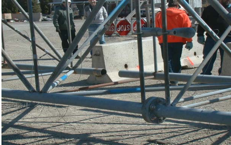
Figure 4. Sign Truss after Cutting the Bottom Chord Member.
