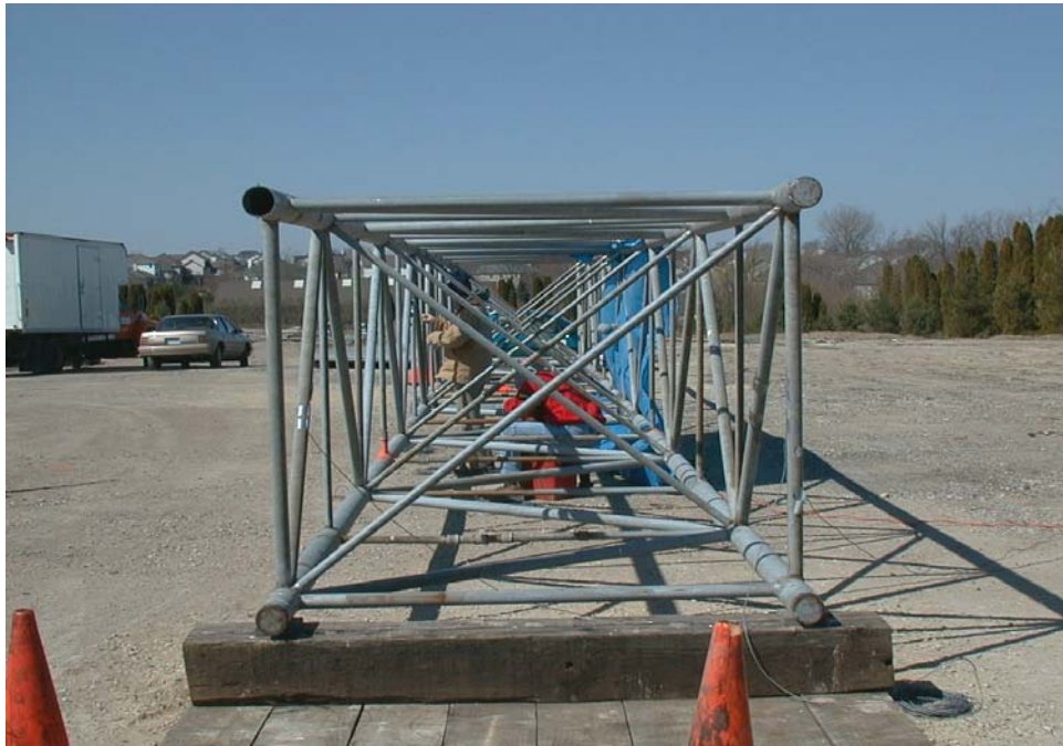
b. Side View of the Sign Truss Figure 3. Experimental Setup.
