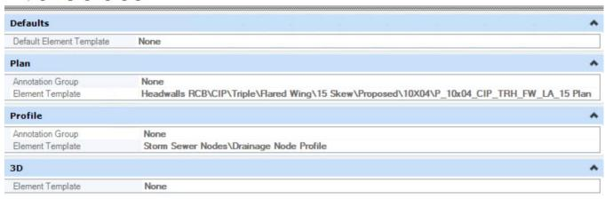
The pipe and culvert feature symbology for the structure profiles are provided under Profile, Conduit, StormWater and Profile, Node, StormWaterNode. These are named the same as the features. Each symbology specifies an element template for the Profile.
