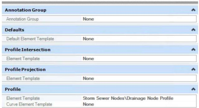
The pipe and culvert feature symbology for the solid category are provided under Solid, Conduit, StormWater and Solid, Node, StormWaterNode. These are named similar to the features. Each symbology specifies an element template for 3D modeling.
