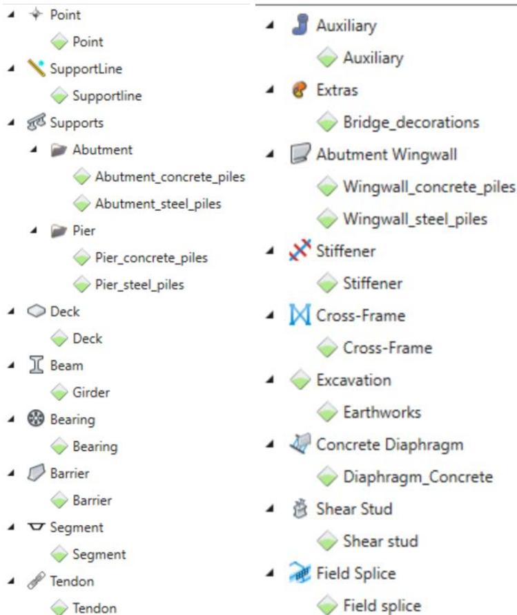
The feature symbology provided through the element templates and levels used are provided in the same dgnlib file.
