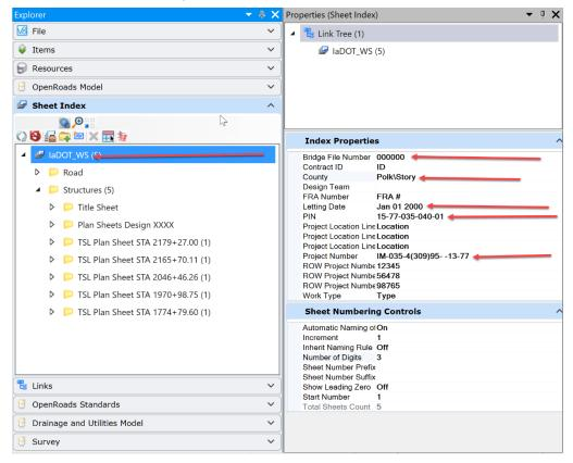
Next, set the text fields that are design number specific for each structure. Select the folder created earlier for each structure in Project Explorer so that it is highlighted and open the Folder Properties.
