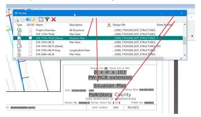
**Note:** If all the values that are entered are not reflecting the same data on the sheet, use the Update All Fields tool. This will reread all the assigned text fields.
