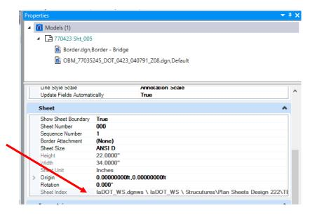
Right clicking on the Sheet Model it can be removed from the Sheet Index, if desired. Sheet Models may also be removed from the Sheet Index through the Sheet Index Explorer.
