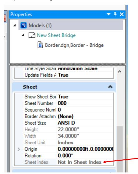
If the Sheet Model was in a Sheet Index then the Remove from Sheet Index option would be selectable.
