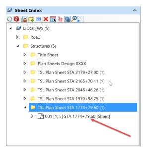
Next, set the Index Properties at the index level. Click on the **IaDOT\_WS** in the Sheet Index Explorer so that it is highlighted and open the Properties. Set the Bridge File Number, County, Letting Date, PIN Number and Project Number. Completing these values will fill out the corresponding text fields in the Border and Title Block of the plan sheet, as well as the corresponding text fields on the Title Sheet.
