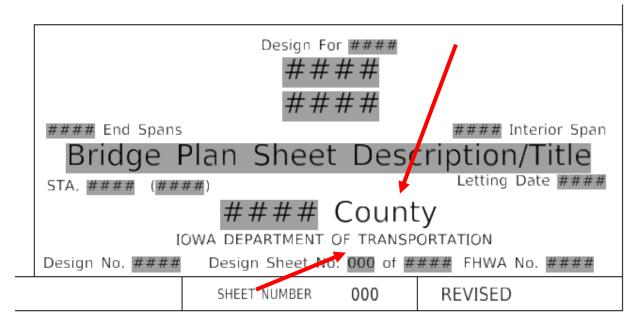
The **Plan Sheet Description** and **Design Sheet No.** text fields are linked to the model properties of the sheet model.
