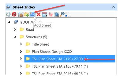
The Add Sheet dialog box will open. Browse to and select the DGN file the sheet is in thru the Select tab.
