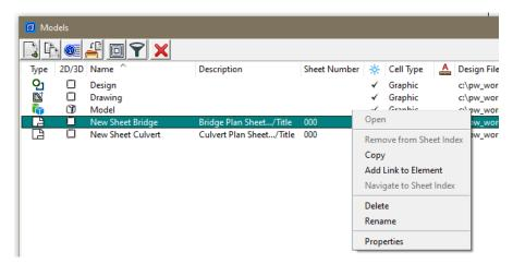
The image below shows the Sheet Model is in a Sheet Index.
