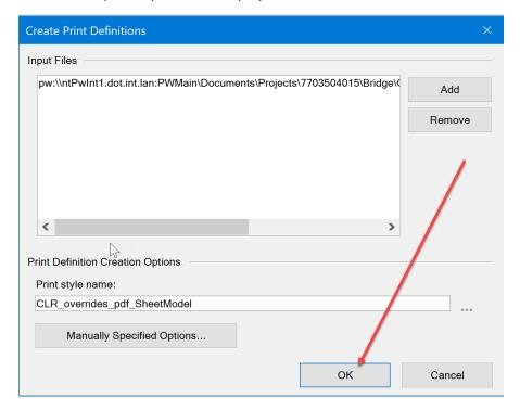
After the Print Organizer compiles the sheets with the model name output, adjust the print property setting for rasters. Currently the print styles are set to print raster images in grayscale. This will need changed in the Properties of the print styles to have the raster images print in color.
