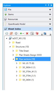
Next, set the Index Properties at the index level. Click on the **IaDOT\_WS** in the Sheet Index Explorer to highlight and open the Properties window.
