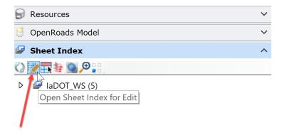
Next, add the folders that the sheets will reside in. Typically, the process is to create a folder for the Pipe sections. Then make subfolders for each cross-section group, alignment.
