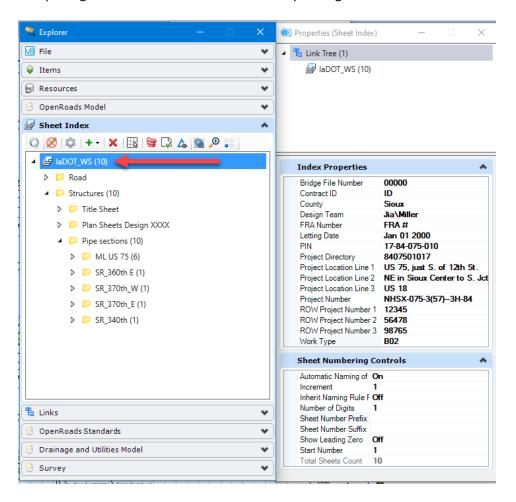
Next, set the text fields that are cross section specific for each cross-section group. To do this, select the folder created earlier for each cross section group in Project Explorer to highlight and open the Folder Properties.
