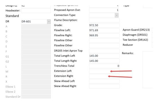
The next two fields are for if the structure is skewed, enter the degree of the angle of the skew in the appropriate field Right or Left.
