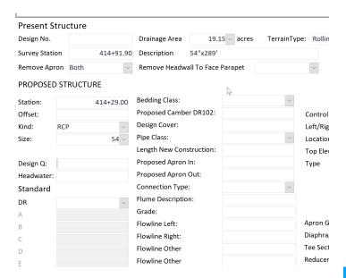
The Next field is the Design Q. Obtain the value from the ICH program that is used to determine the size of the proposed structure. This comes from the lowa Runoff Chart.
