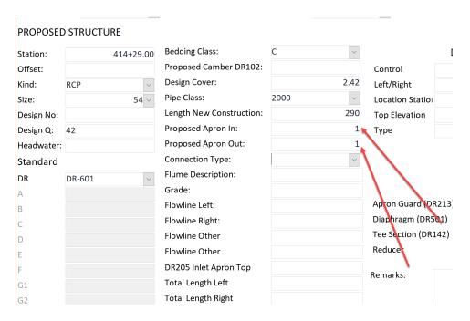
The next field, Connection Type, is for indicating if the design requires a connection type, either a <u>DR-122</u> or <u>DR-141</u>. Select the correct standard and the additional field will appear for the corresponding information for that standard. This will not be used for this design.
