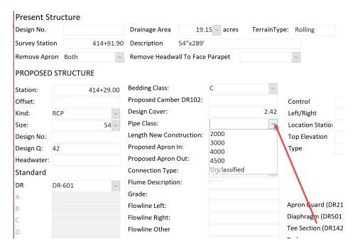
Next, enter the Length New Construction value. This is the total length from connection point of inlet apron to connection point of outlet apron. For the example it will be 290'.
