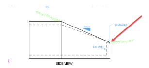
The next two fields are to report on the Total Length Left and the Total Length Right. This is the distance from center line to end of the apron.
