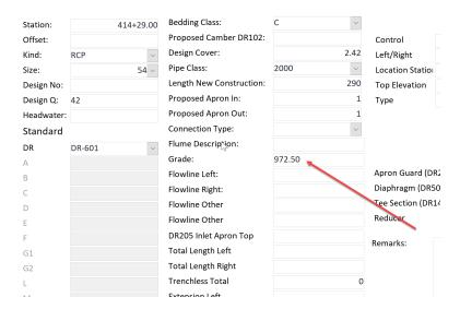
The next 2 fields will be Flowline Left and Flowline Right. This is the elevation of the flowline at the end of the pipe apron.
