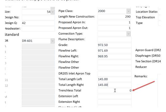
The next two fields are for if the design is to extend the existing structure. Enter the total distance in the direction of the extension that is to be constructed.
