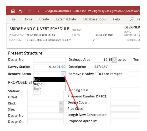
If the structure is an RCB, click on the pulldown on the Remove Headwall field. This will provide 3 options, Left, Right and Both. If the RCB is being extended, select the end that is being extended. However, if the RCB is being replaced select Both.
