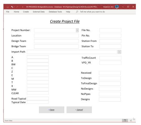
The first step to start a new project is to import the Survey Records into the new project. Click on the magnifying glass next to the Import Path field.
