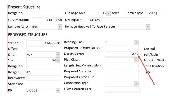
Next, decide what class of pipe is used for this design. This is determined by the design cover and Bedding Class. Refer to the <u>DR-104</u> to verify. Use 2000 for this example.
