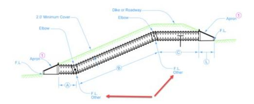
The next field, DR205 Inlet Apron Top, is for the elevation at the top of the end wall of a <u>DR-205</u>. If this apron is used in the design, enter the elevation here.
