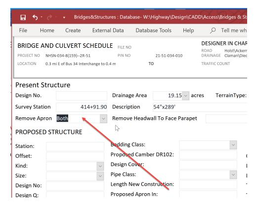
Next, fill out the Station of the Proposed Structure. This is the station value that is the intersection point at the centerline of the Proposed Structure and the centerline of the design alignment. For this example, it will be 414+29.00.
