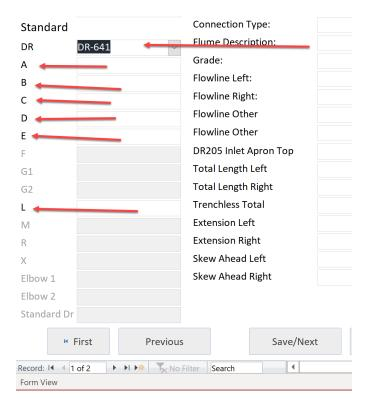
**Note:** When entering a <u>DR-641</u> use two records in the database. One for the concrete or RCP portion of the structure and one for the CMP or plastic letdown section of the structure. Enter RCP portion on the first record with all special dimensions. Then just the letdown dimensions on the second record. This will allow the structure to be tabulated correctly.
