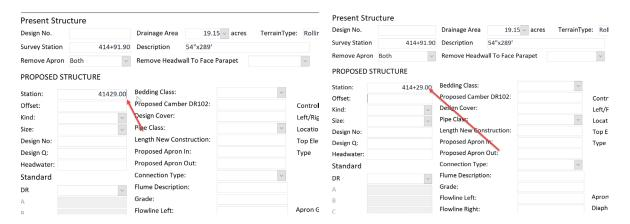
The next field is Offset field. This is used if the structure is on a divided highway. This will be the distance from the mainline centerline to the Base Line as described in the standards.
