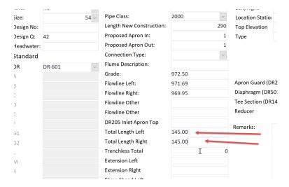
The next field is for reporting the Trenchless Total. This will refer to a pipe that requires to be jacked in place during installation as opposed to being replaced by cut and cover. This field is to enter the total distance of that pipe that is to be jacked.
