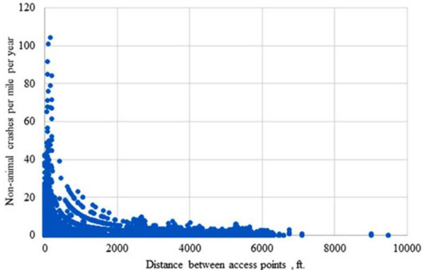
On two-lane highways, the crash rates have a similar shape to multi-lane highways but have a lower crash frequency. For two-lane highways, access spacing distance was shown to have persistent effects at distances of up to 2,640 feet. As spacing distance was reduced, crashes increased by 17.2% for distances up to 1,320 ft.
