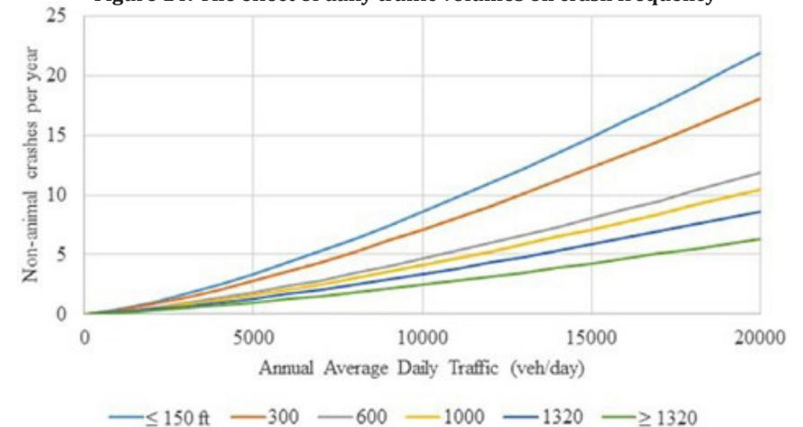
For each signalized intersection, crashes in a multilane segment increased by 59% as compared to the average values shown in the above curves. Where segments included two traffic signals, the crash risk should double as compared to segments without signals.
