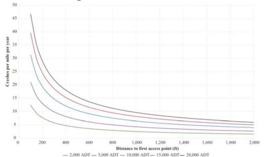
Following the crossroad study, a similar analysis was conducted for the expressway transition areas. This is where a motorist is traveling along an expressway through an interchange area providing a freeway type experience, and then arriving at a signalized or non-signalized intersection on the far side of the interchange.
