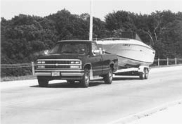
**Hitch Location** The closer you can get the hitch to the rear axle of the towing vehicle, the better your trailer will ride. Try to keep the hitch up against the bumper. Do not put too much stress on the bumper without bracing it to the frame.
