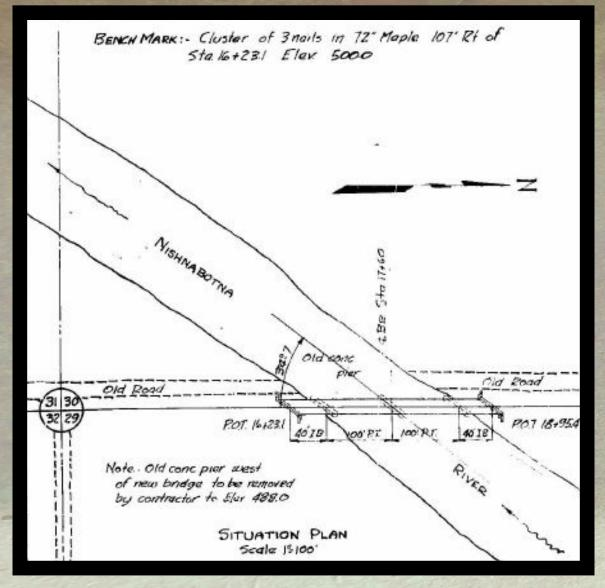
Above: Situation plan from the Iowa Highway Commission Standard Design Plans for the Nishnabotna River Bridge. These plans depict the adjustments engineers made to accomodate the river channel and flow patterns.
