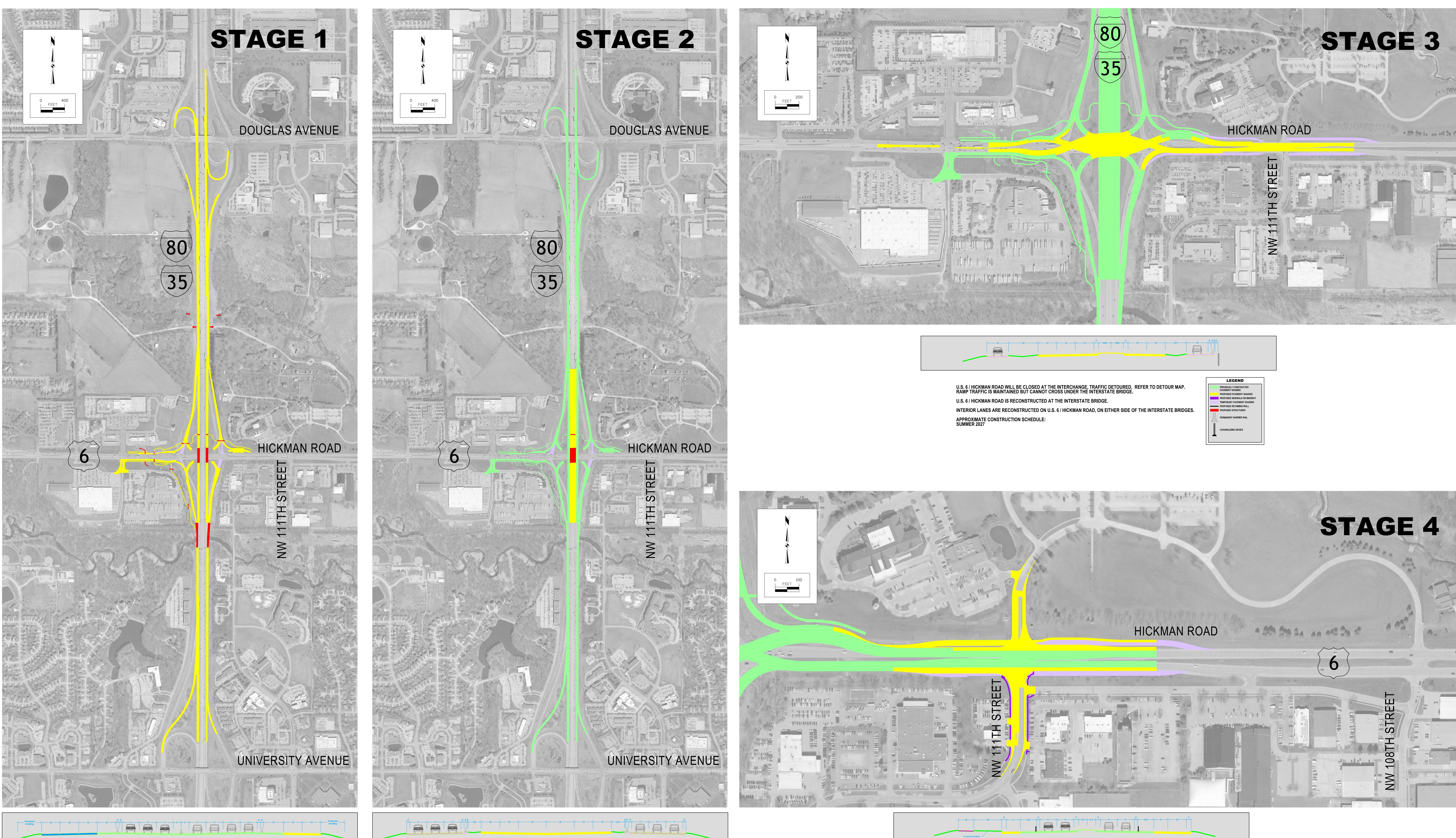
INTERSTATE TRAFFIC SHIFTS TO UTILIZE INTERIOR LANES, THREE LANES IN EACH DIRECTION MAINTAINED AT ALL TIMES. HICKMAN ROAD REMAINS OPEN TO TRAFFIC, TWO LANES IN EACH DIRECTION MAINTAINED AT ALL TIMES. GRADE AND PAVE NEW OUTSIDE LANES ON INTERSTATE 35/80. GRADE NEW OUTSIDE LANES ON U.S. 6 / HICKMAN ROAD. WIDEN INTERSTATE BRIDGE OVER WALNUT CREEK. PARTIALLY DEMOLISH EXISTING INTERSTATE BRIDGES AND PARTIALLY CONSTRUCT NEW INTERSTATE BRIDGES OVER U.S. 6 / HICKMAN ROAD.
