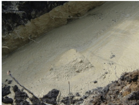
Figure D.45. Drilling fluid close-up showing texture
