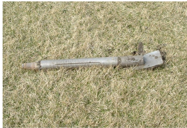
Figure D.39. Five inch diameter pilot bore drill bit
