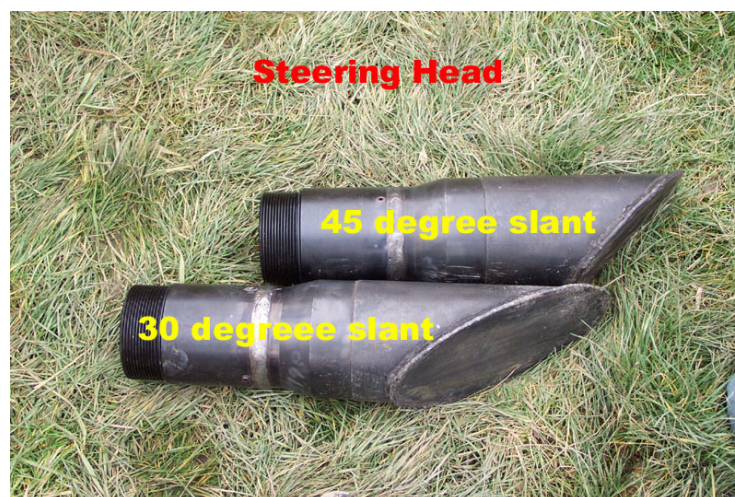
Figure 2.20. PTMT steering heads (Purdue University)
