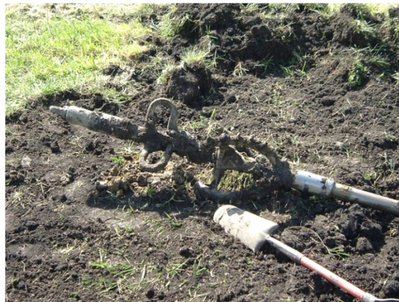
Figure 4.123. Reamer (16-inch diameter) attached to drill string
