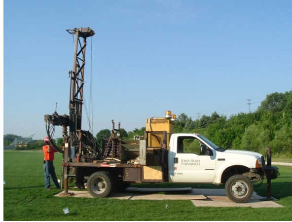
Figure 4.44. Drill rig used by research team to recover soil samples
