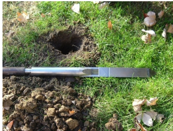
Figure 4.65. Push-in pressure cell before installation
