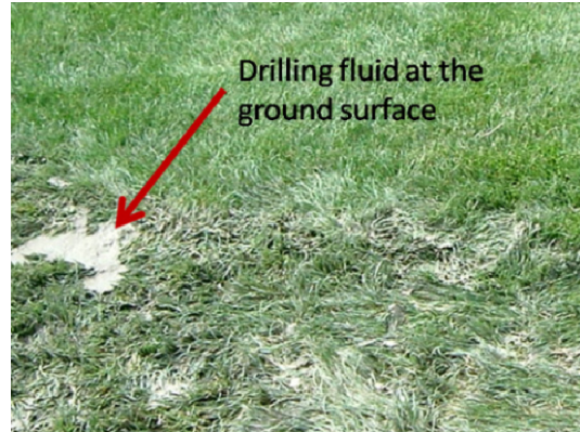
Figure 4.39. Edge of frac-out region with drilling fluid at the ground surface
