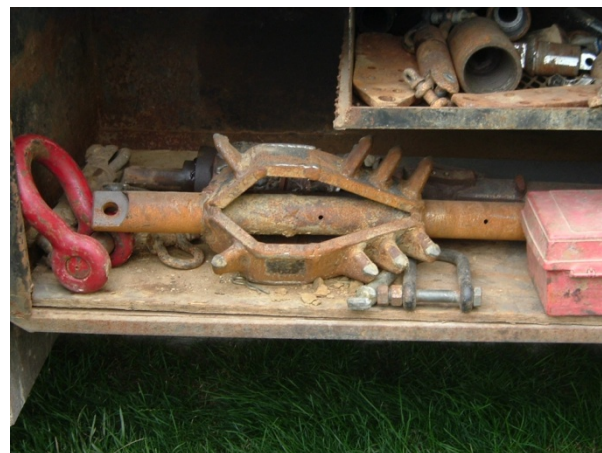
Figure D.23. Fourteen inch diameter reamer
