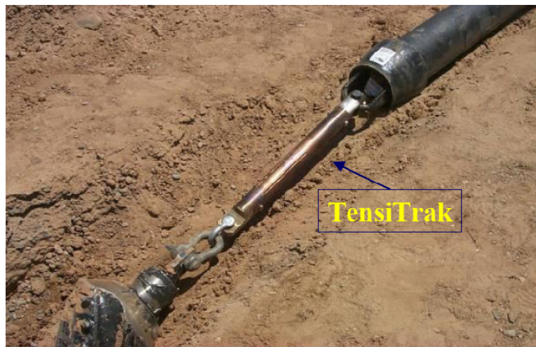
Figure 2.15. Weak-link device (trade name “TensiTrak”) (NASTT 2005)
