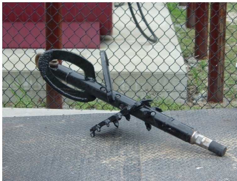
Figure 2.13. Reamer with 14-inch-diameter
