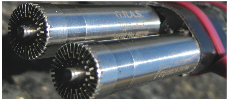
Figure 1. Sound intensity probe used for OBSI testing showing two 1/2 in. microphones (photo does not show foam windscreen required during testing)
