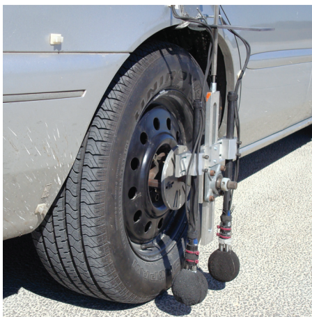
Figure 3. OBSI configurations with a single sound intensity probe (top) and dual probe (bottom)
