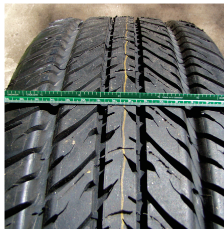
Figure 4. Standard tires used in CPSCP OBSI Testing – Goodyear Aquatred 3 (left) and ASTM F 2493 SRTT (right)
