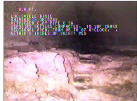
Photo: OH15269_OH15266124326_05112009_A.JPG, VCR No.: FLOOD WALL#2, 01:42:36 0FT, Deposits Settled Compacted, 15 %of cross sectional area, from 05 to 07 o'clock, within 8 inches of joint: YES
