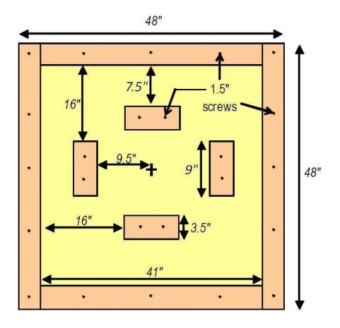
Figure 2 Apparatus – Top View (Frame)
