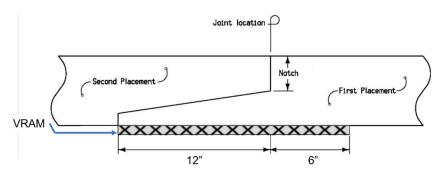
Figure 2: Example illustration of VRAM with a compacted notched-wedge joint. Drawing not to scale. Cross sections will vary. Refer to plans.
