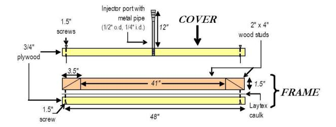
Figure 1 Apparatus - Side View
