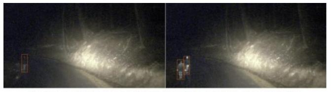
Perception of foggy night using regular camera (left) where only one of the two pedestrians is slightly visible vs after Plus's proprietary thermal augmentation (right)
