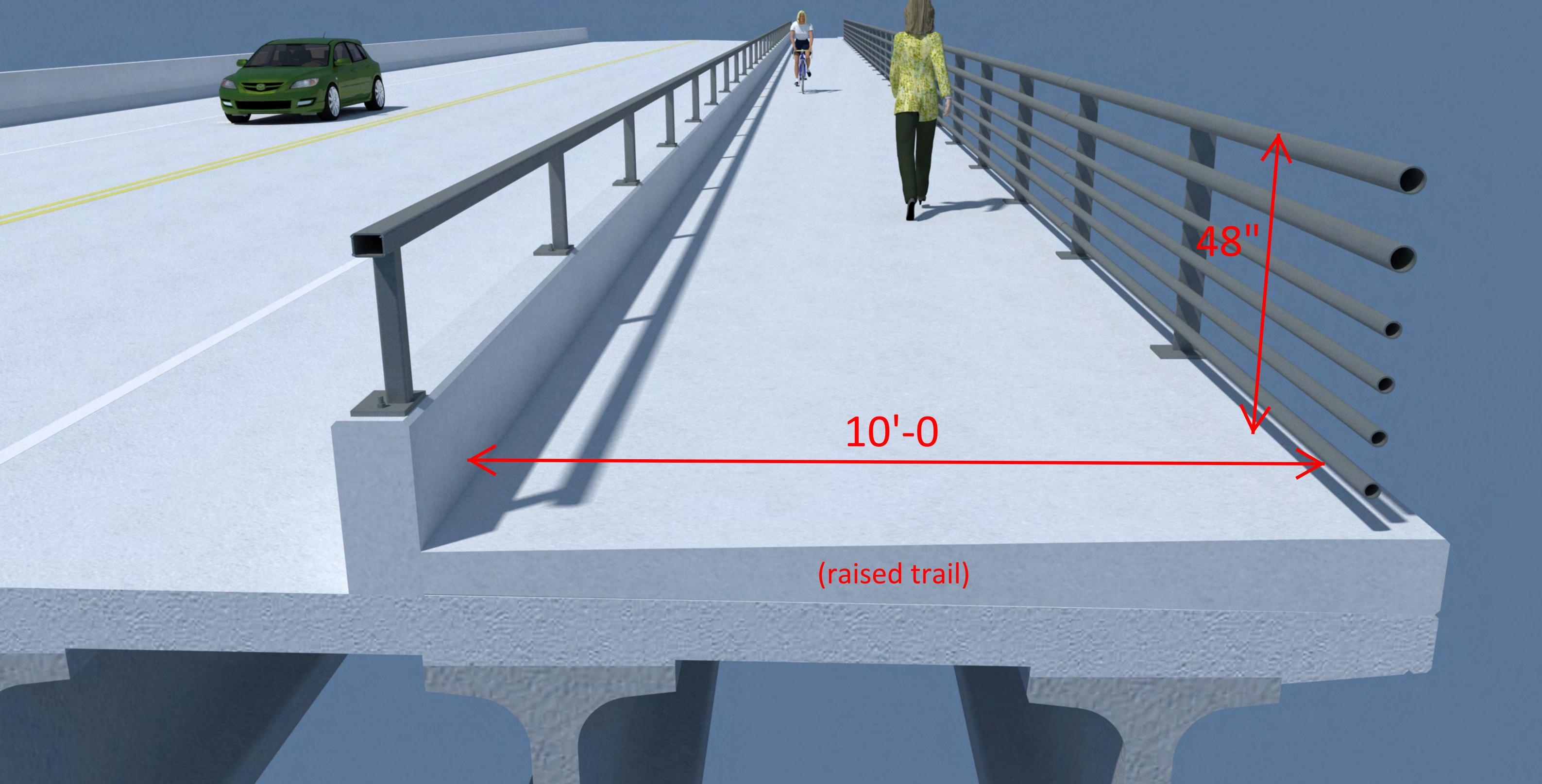
Shared Use Paths on Vehicular Bridges: Bike Plan Guidance (min. railing hgt.)
