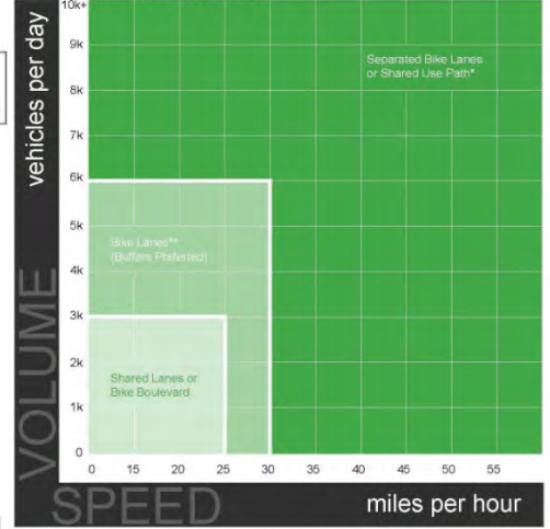
FIGURE 3: BICYCLE FACILITY SELECTION
