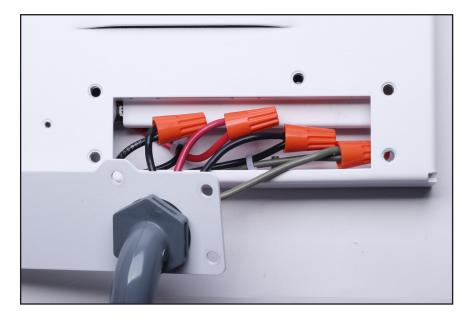
Attach Access Plate to PMG Sign and tighten screws.
