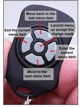
Figure 33 Note: Each Key Fob is paired with an individual PMG. Take care to keep the two together.
