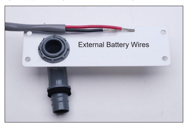
Feed the External Solar Wires and External Battery Wires through elbow as shown.
