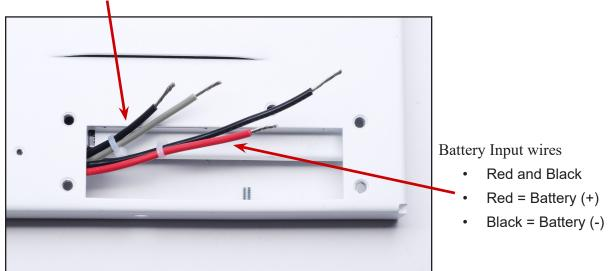
Using appropriately sized wire nuts, twist and lock:
