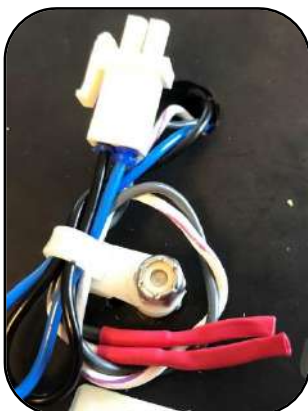
Optional: If present, disconnect strobe connectors.
