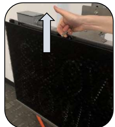
Lift window retainer clip
