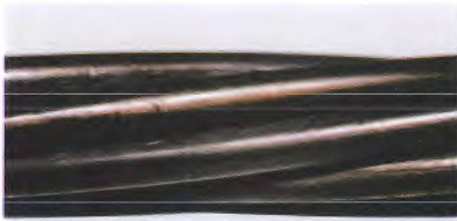
Photo 1. Strand surface before cleaning.
