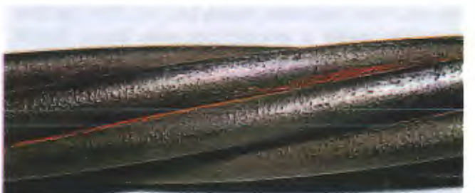
Photo 3A. Strand surface after cleaning.
