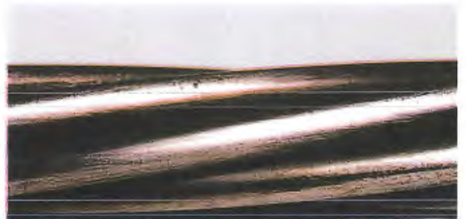
Photo 1A. Strand surface after cleaning.
