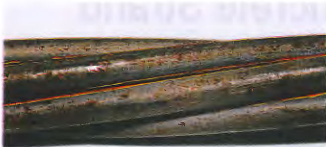
Photo 1. Strand surface before cleaning.
