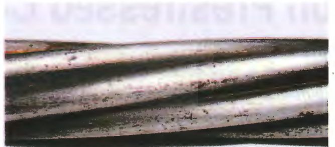
Photo 1A. Strand surface after cleaning.
