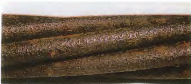
Photo 5A. Strand surface after cleaning.
