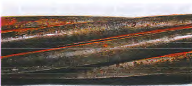
Photo 2. Strand surface before cleaning.
