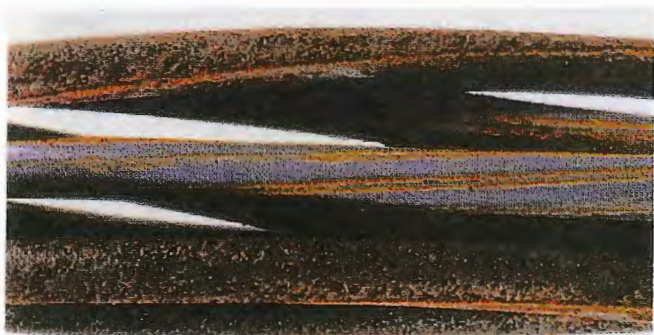
Photo 8. Strand surface before cleaning.
