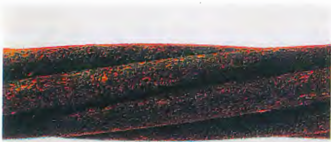
Photo 6. Strand surface before cleaning.
