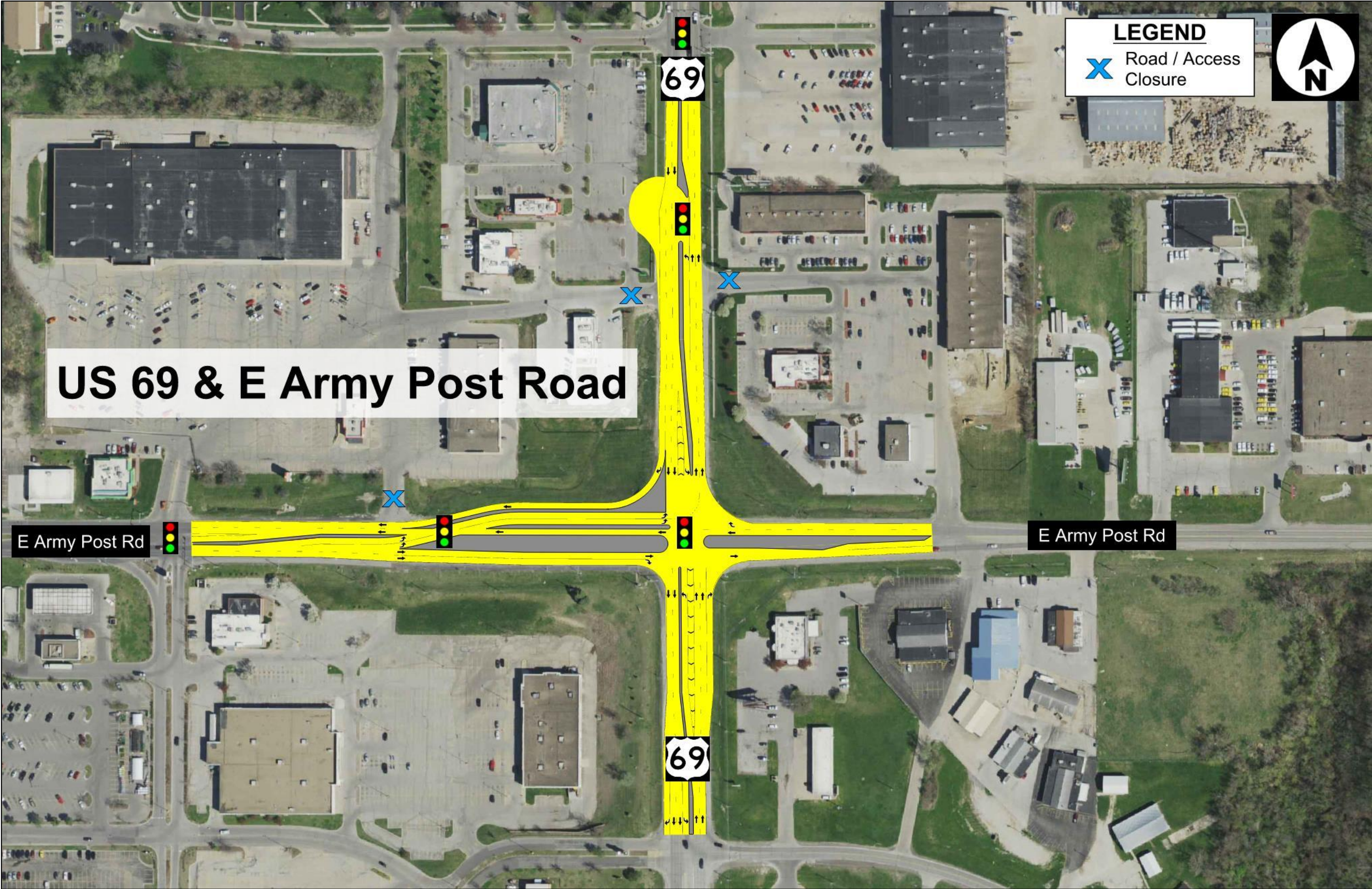
Figure 11. US 69 & E Army Post Road Schematic Alternative (DLT Intersection with MUT on North Leg)
