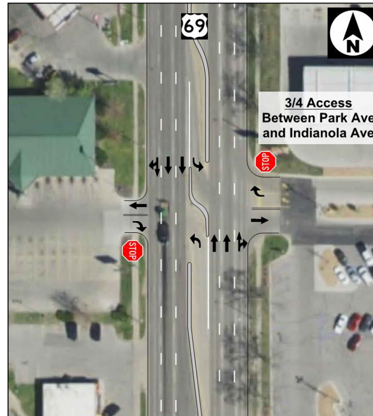
Figure 31. ¾ Access Between E Park Avenue & Indianola Avenue (Existing)
